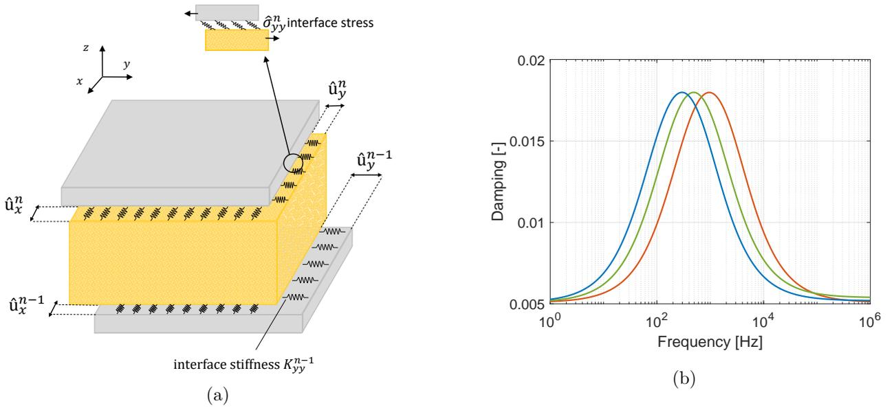
Figure 1: (a) Typical three-layered composite with a soft and thick core and illustration of the sliding with the generated interface stiffness, (b) Equivalent loss factor with perfect interfaces (—) and with imperfect interfaces: one imperfect interface (—), two imperfect interfaces (—).
