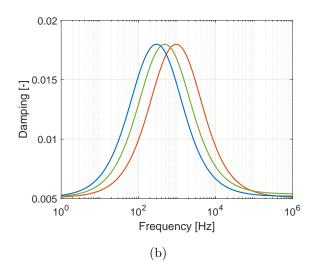
Figure 1: (a) Typical three-layered composite with a soft and thick core and illustration of the sliding with the generated interface stiffness, (b) Equivalent loss factor with perfect interfaces (-) and with imperfect interfaces: one imperfect interface (-), two imperfect interfaces (-).
