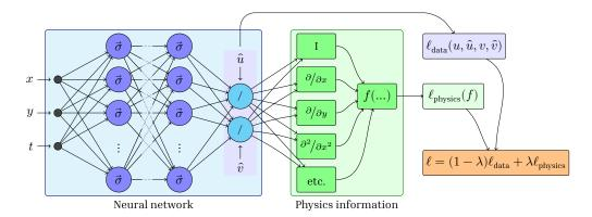
Figure 3.5: Schematic representation of a physics-informed neural network with inputs x,y, and t; outputs  $\hat{u}$  and  $\hat{v}$ . Using automatic gradient calculation we can differentiate the neural network by its input variables and construct a physics error function f(). Consequently, the loss function,  $\ell$ , involves a loss term for the data ( $\ell_{\rm data}$ ) and a loss term for the physics function ( $\ell_{\rm physics}$ ). Source: de Wolff et al. 2021b.
