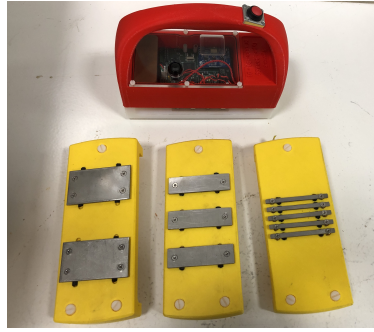
Figure 3: Capacitive measurement system with the four different electrode arrays. Yellow arrays from left to right are LE1, ME1, SE1 and white array connected to the red system is SE2 (see text for details).
