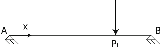
Fig. 3 An elastic rope supporting a load at a position x = X
