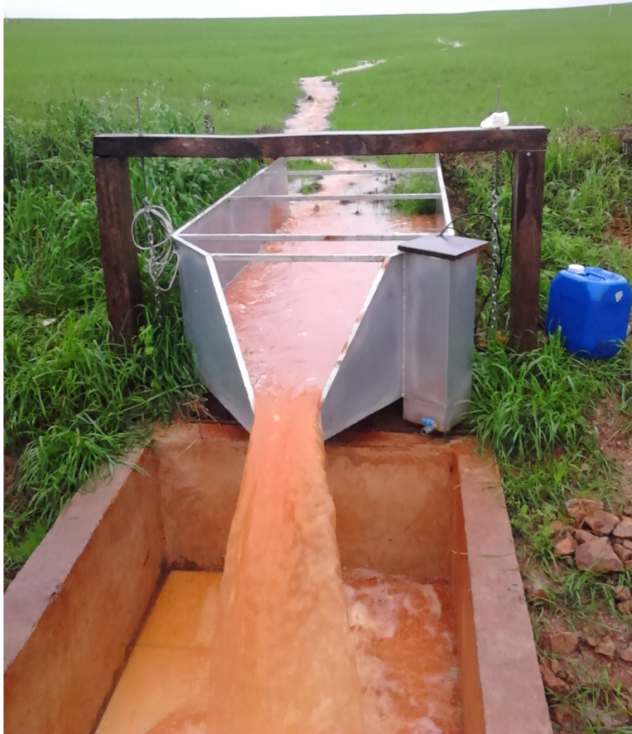
Figure 3. H-flume for monitoring the flow rates installed in the lower part of the catchments and macroplots.
