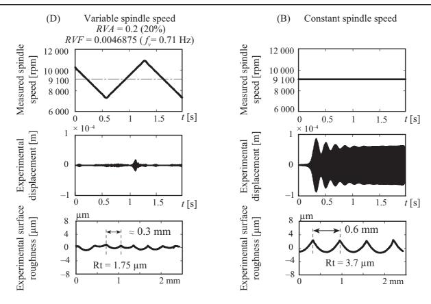
Figure 9: Chatter suppression by spindle speed variation ( $A_p = 1 \text{ mm}$  and  $N_0 = 9100 \text{ rpm}$ ).
