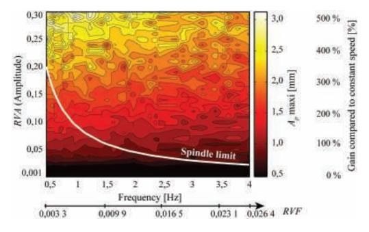
Figure 5: Parametric study for sinusoidal shape ( $N_0 = 9100$  rpm and  $A_e = 2$  mm).
