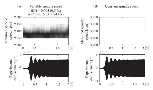
Figure 7: Two machining unstable ( $A_p = 1 \text{ mm}$  and  $N_0 = 9100 \text{ rpm}$ ).
