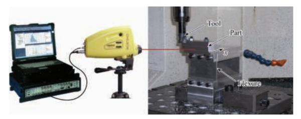
Figure 6: Experimental set-up.
