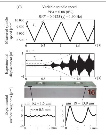
Figure 8: Analysis of an unstable machining ( $A_p = 1 \text{ mm}$  and  $N_0 = 9100 \text{ rpm}$ ).
