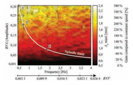
Figure 4: Parametric study for triangular shape ( $N_0 = 9100$  rpm and  $A_e = 2$  mm).
