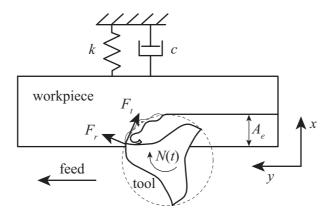
Figure 2: Mechanical model of the milling process.
