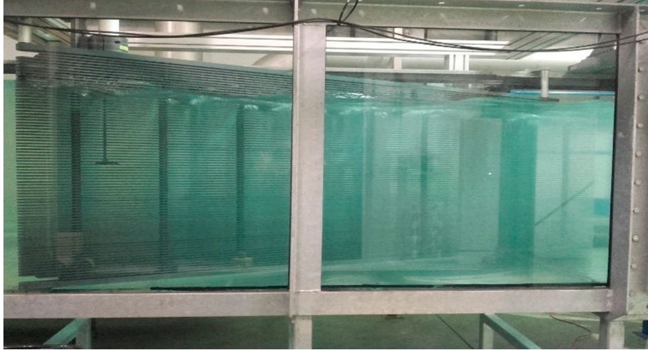
Figure 2 Angled trash rack with horizontal bars
