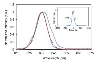
**Fig. 5.** Spectra of the seed pulses (dotted red curve) and the compressed pulses (solid blue curve). Spectrum of the free running cavity-dumped amplifier (solid grey curve). Inset: Single-shot autocorrelation trace of the compressed pulses. The FWHM is 154 fs, corresponding to a pulse duration of 100 fs.
