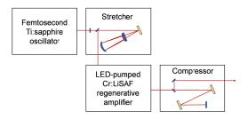
**Fig. 1.** Schematic of the chirped pulse amplification using a Cr:LiSAF regenerative amplifier. The oscillator produces 90 fs pulses at 835 nm. The Cr:LiSAF regenerative amplifier is pumped by LEDs and operates at 10 Hz. The pulses are temporally stretched (up to 100 ps) and recompressed using grating-based pulse stretcher and compressor.
