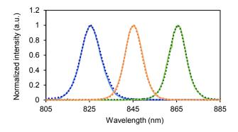
**Fig. 7.** Spectra of the seed pulses (dotted curves) and the amplified pulses (solid curves) between 825 nm and 865 nm.
