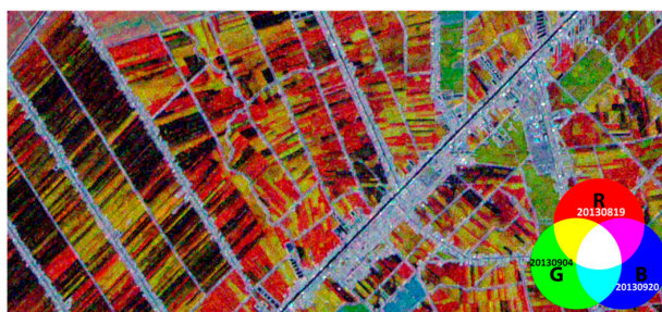
Figure 6. Example of RGB combinations of different dates (R: 19/08/2013, G: 04/09/2013, B: 20/09/2013) from CSK images, HH polarization over rice fields in the An Giang Province.
