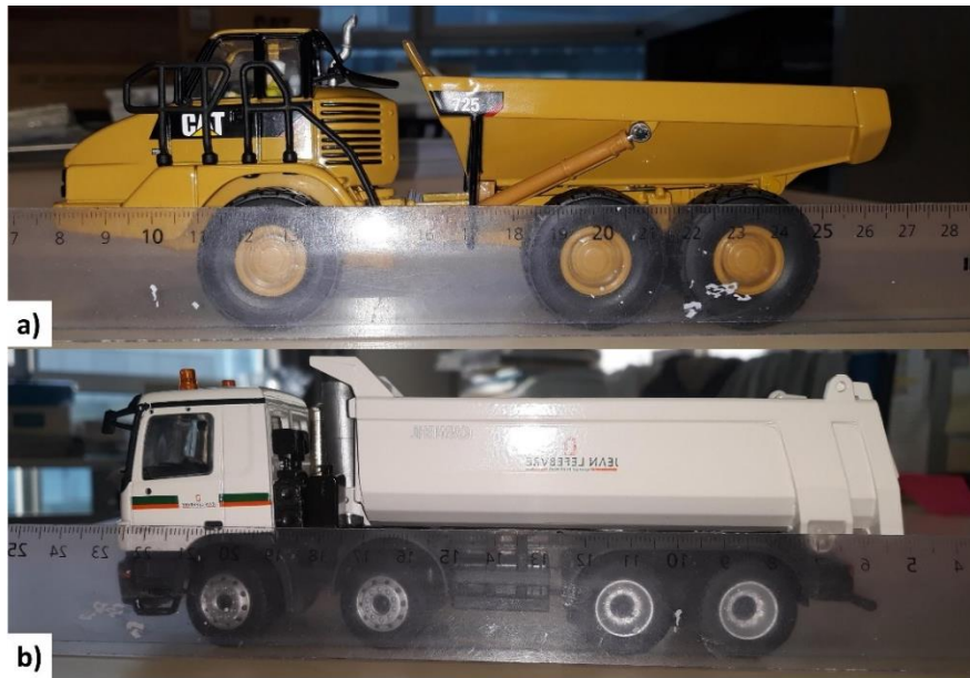
Figure 5. Wind tunnel scale model of a) Caterpillar articulated dump truck and b) Mercedes 8x4 cab-over truck.
