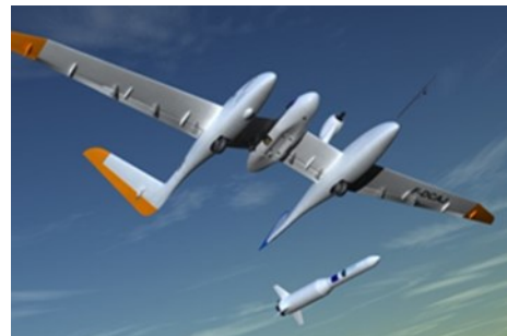
Fig. 2 Artist's view of the small scale demonstrator EOLE releasing a rocket mock-up
