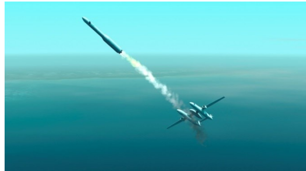
Fig. 1 Artist's view of the ALTAIR system after release of the rocket by the carrier
