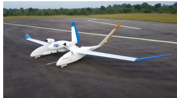
Fig. 14 : EOLE demonstrator equipped with a launcher mock-up at CSG airfield
