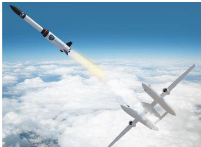
Figure 2. Artist's view of the ALTAIR system after release of the rocket by the carrier
