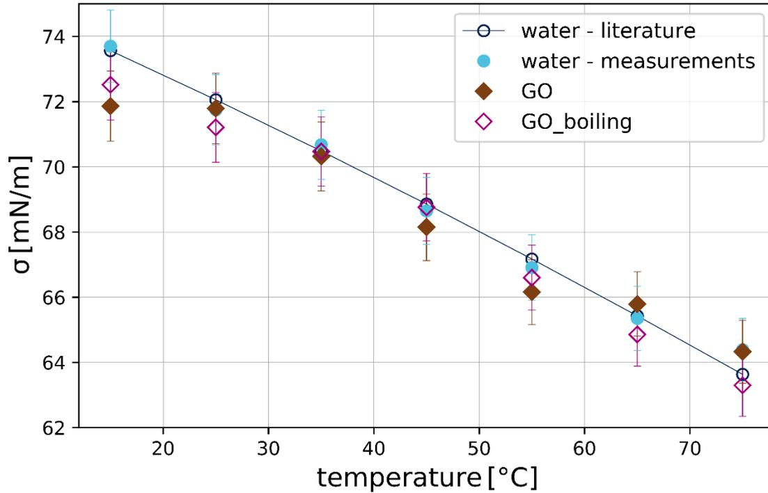
Fig. 4. Surface tension of nanofluid based on graphene oxide flakes in comparison with water: fresh graphene oxide nanofluid before (*GO*) and after (*GO\_boiling*) experimental research in the thermosyphon. Uncertainty bars represent standard deviation.
