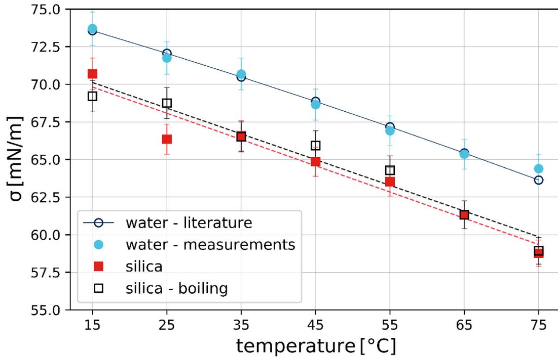
Fig. 3. Surface tension of silica nanofluid in comparison with water: fresh silica nanofluid before (*silica*) and after (*silica - boiling*) experimental research in the thermosyphon. *Water – measurements* are the results obtaining during calibration of the device with distilled water and are compared with literature values (*water – literature*) [60]. Uncertainty bars represent standard deviation.
