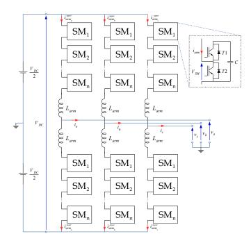
Fig. 1. Structure of the MMC
