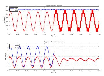
Fig. 11. Input voltage and HIL estimated output voltage and currents. Load switched out at 7.5s
