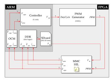
Fig. 5. MMC IP working as HIL
