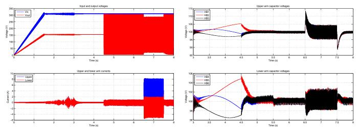
Fig. 6. Input voltage and HIL estimated output voltage and currents - Complete simulation
