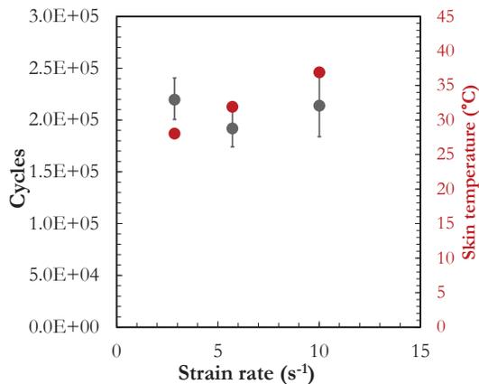
Figure 9: Effect of the testing frequency on the fatigue life based on the end-of-life criterion in the case of a non relaxing test defined by  $\varepsilon_{mean} = 322\%$  and  $\varepsilon_{amp} = 72\%$  corresponding to a load ratio  $R_\varepsilon = 0.64$ .
