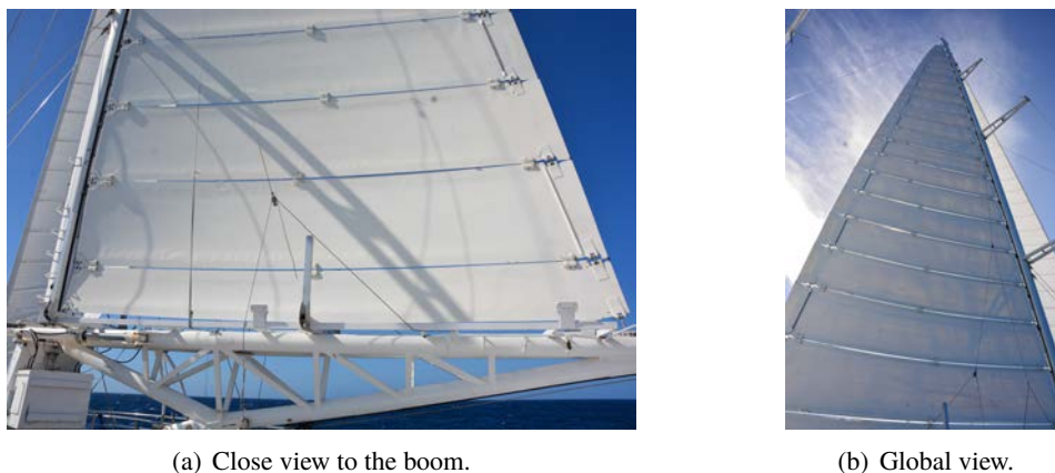
Figure 1: Semi-rigid prototype mainsail hoisted on the “ Ponant ” yacht.
