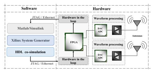
Figure 13. Co-simulation platform.
