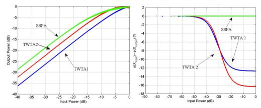
**Figure 2.** HPA non-linear response for amplitude (**left**) and phase (**right**). TWTA1:  $\alpha_{||} = 2$ ,  $\beta_{||} = 1$ ,  $\alpha_{PM} = 4$ ,  $\beta_{PM} = 9$ , TWTA2:  $\alpha_{||} = 3$ ,  $\beta_{||} = 2$ ,  $\alpha_{PM} = 2$ ,  $\beta_{PM} = 7$ , SSPA: NEC GaAs [10].
