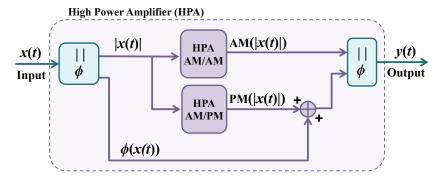
Figure 1. HPA's operating principle.
