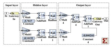
Figure 7. Implementation for NN AM/AM SSPA pre-distorter.
