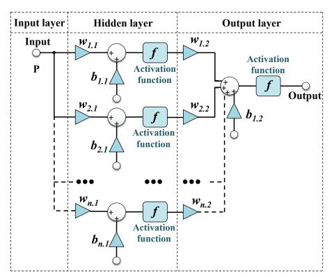
Figure 5. Multilayer perceptrons neural networks pre-distorter.
