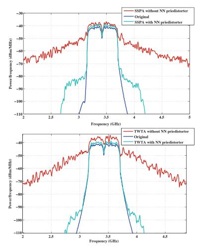
**Figure 18.** Power Spectral Density: without NN pre-distorter and with implemented NN pre-distorter on Xilinx for both TWTA and SSPA.
