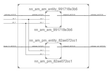
Figure 8. RTL Schematic for NN TWTA and SSPA pre-distorters.
