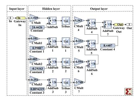
Figure 6. Implementation for NN AM/AM TWTA pre-distorter.
