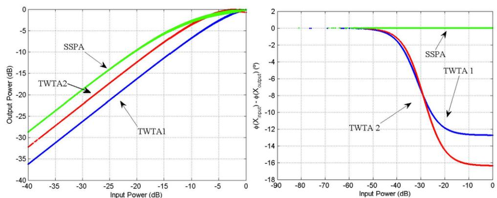
**Figure 2.** HPA non-linear response for amplitude (left) and phase (right). TWT1:  $\alpha_{||} = 2, \beta_{||} = 1, \alpha_{PM} = 4, \beta_{PM} = 9$ , TWT2:  $\alpha_{||} = 3, \beta_{||} = 2, \alpha_{PM} = 2, \beta_{PM} = 7$ , SSPA: NEC GaAs [10].
