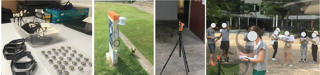
Figure 5: From left: sensor calibration in indoor laboratory; Hobo MX2302 temperature and humidity logger installed on site with a radiation shield; Kestrel 5400 Heat Stress Tracker at survey stations; and participants answering survey questions while wearing modified wearable devices. We ensured that the participants have been in Singapore for the week preceding the experiment (i.e. no overseas travels to hotter or colder climates that can affect their thermal sensation) and are well-rested to undertake a walk on flat terrain (40-50 minutes duration). Fixed environmental sensors are placed at the height of wearables at wrist (1.1 – 1.2 m).
