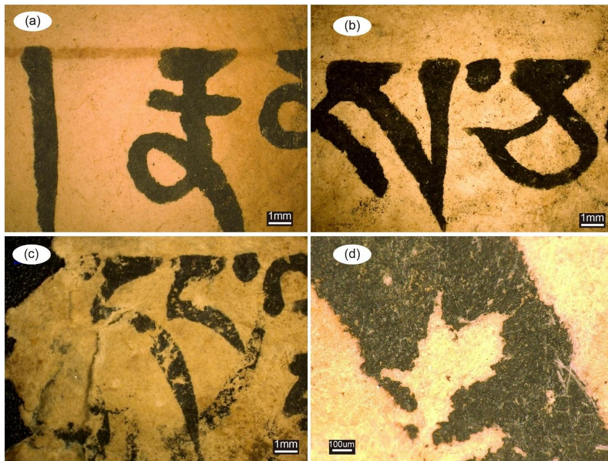
284 285 Figure.3 the state of the fragment under the microscopy: (a) the transverse scribal guidelines, (b) the ink diffusion state, (c) 286 and (d) the agglomeration and caking off the ink on the paper surface.
