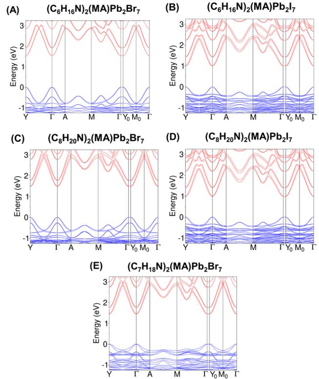
**Figure 8.** DFT computed band structures of (A) C6BrN2, (B) C6I2, (C) C8BrN2, (D) C8I2, and (E) C7BrN2. The valence and conduction bands are depicted in blue and red, respectively. All compounds exhibit strong dispersion within the layers and flat dispersion in the stacking direction.
