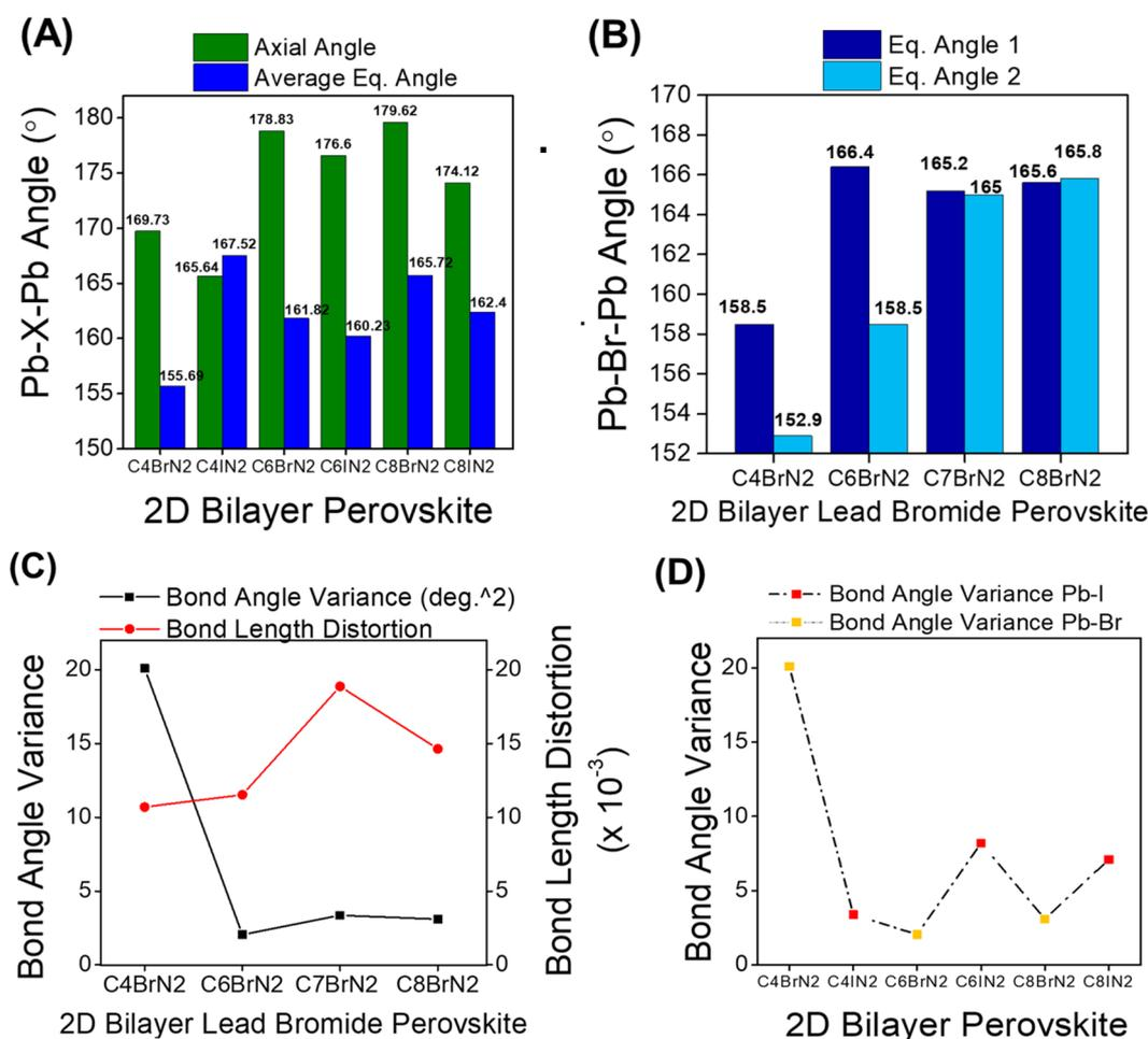
**Figure 6.** (A) Average axial and equatorial Pb–Br–Pb angles, (B) equatorial Pb–Br–Pb angles, and (C) bond angle variance and bond length distortion of C4BrN2, C6BrN2, C7BrN2, and C8BrN2. (D) Bond angle variance of C4BrN2, C6BrN2, and C8BrN2 versus C4IN2, C6IN2, and C8IN2.
