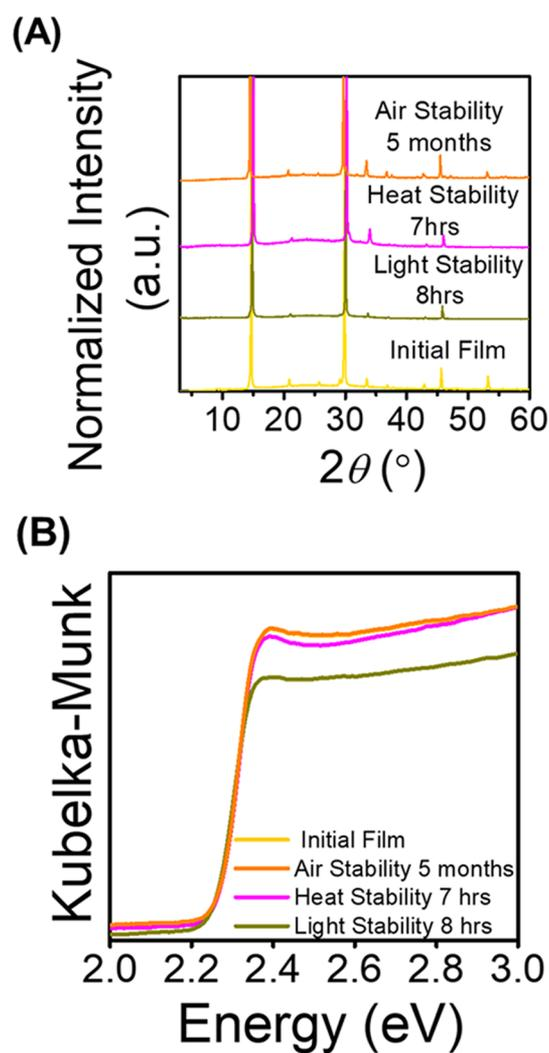
**Figure 12.** (A) Powder X-ray diffraction patterns and (B) absorption spectra of thin films of MAPbBr<sub>3</sub>, before stability testing (yellow) and afterward from air stability testing after 5 months (orange), heat stability testing after 7 h total (pink), and light stability testing after 8 h total (green).
