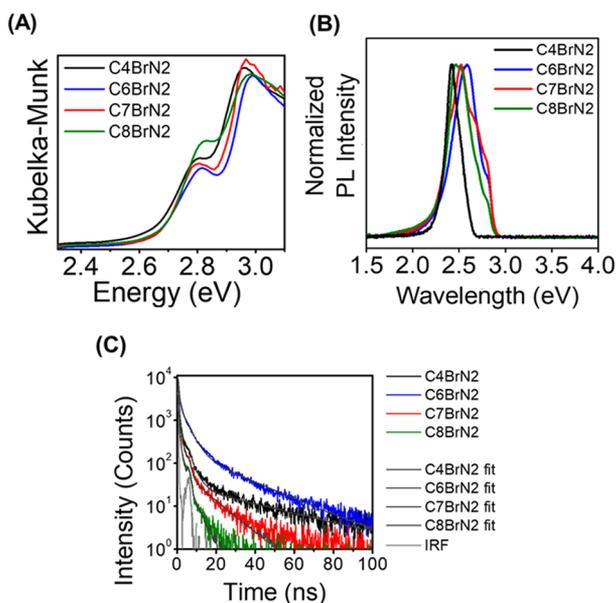
**Figure 7.** (A) Optical absorption spectra, (B) steady-state PL emission spectra collected with a long pass filter of 370 nm and excited at 405 nm, and (C) time-resolved PL decays and fitting collected at room temperature of C4BrN2, C6BrN2, C7BrN2, and C8BrN2.
