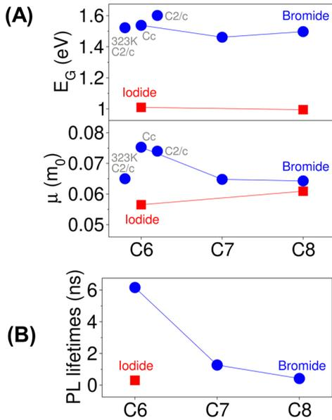
**Figure 9.** (A) Computed bandgaps ( $E_G$ ) and reduced effective masses ( $\mu$ ) for C6BrN2, C7BrN2, and C8BrN2 (blue circles), as well as C6IN2 and C8IN2 (red squares) compounds. In addition to the noncentrosymmetric Cc structure of C6BrN2, the computed bandgaps of the noncentrosymmetric and the 323 K C2/c structures are given. (B) Measured photoluminescence lifetimes for C6BrN2, C7BrN2, C8BrN2 (blue circles), and C6IN2 (red square).
