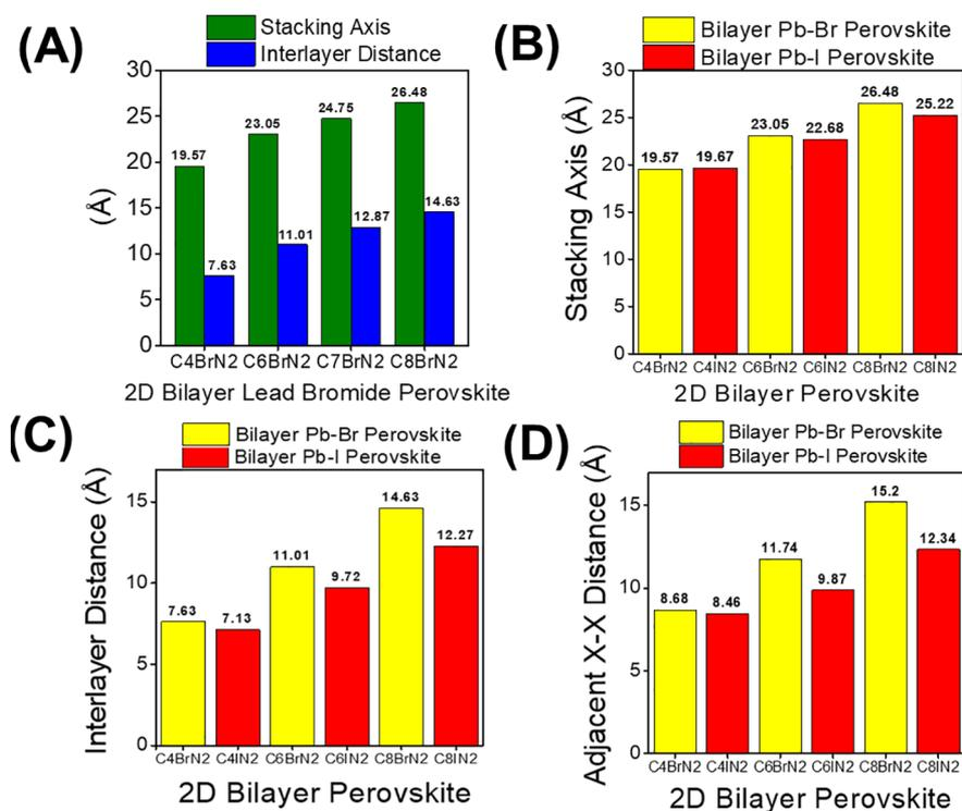
**Figure 3.** (A) Comparison of stacking axis and interlayer distance from crystal structures of 2D lead bromide perovskites C4BrN2, C6BrN2, C7BrN2, and C8BrN2. (B) Comparison of stacking axis, (C) interlayer distance, and (D) adjacent X–X (X = halide) distance from crystal structures of 2D lead bromide perovskites C4BrN2, C6BrN2, and C8BrN2 versus 2D lead iodide perovskites C4IN2, C6IN2, and C8IN2.
