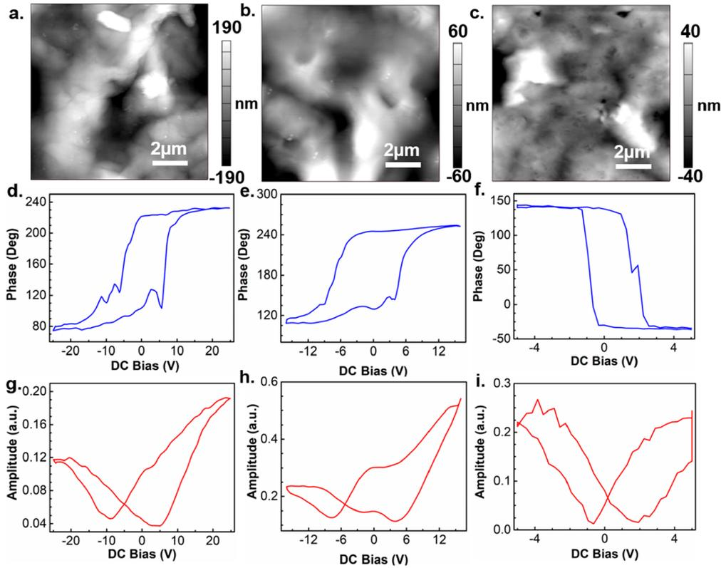
**Figure 14.** (A–C) Surface morphology of the resulting thin film samples of C6BrN2, C7BrN2, and C8BrN2. (D–F) Local response of the phase to the applied DC electrical field. (G–I) Local response of amplitude to the applied DC electrical field.
