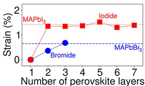
**Figure 10.** In-plane average lattice strain considering the monolayered compounds with C4 spacer as references for bromide (blue circles) and iodide (red squares) compounds. The dashed blue and dotted red lines represent the lattice mismatches with the related MAPbBr<sub>3</sub> and MAPbI<sub>3</sub> compounds, respectively.
