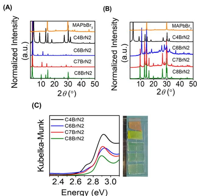
**Figure 11.** Powder X-ray diffraction patterns of thin-films of MAPbBr<sub>3</sub>, C4BrN2, C6BrN2, C7BrN2, and C8BrN2 made from the (A) one-step and (B) hot-casting methods. (C) Absorption spectra of thin films C4BrN2, C6BrN2, C7BrN2, and C8BrN2 alongside picture of thin films.
