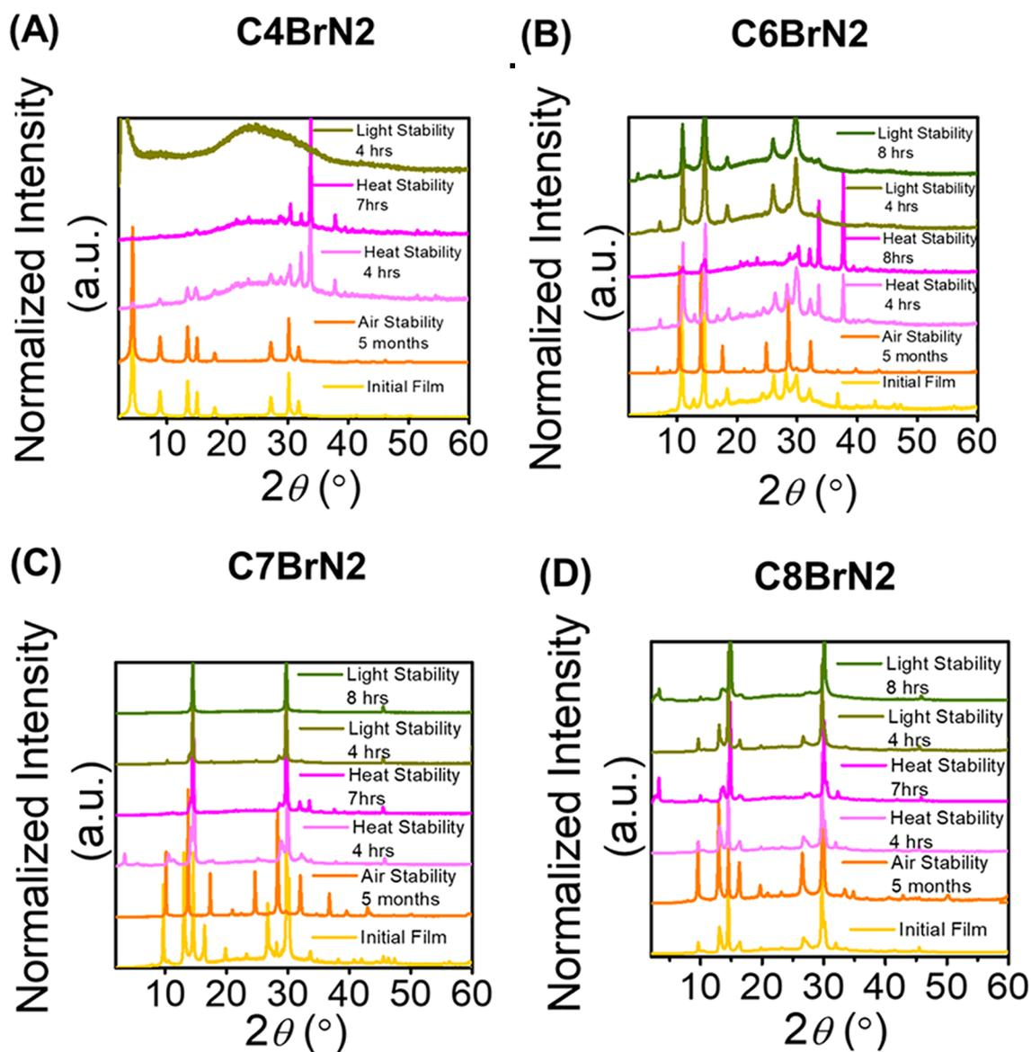
**Figure 13.** Powder X-ray diffraction patterns in ambient conditions, from before and after stability tests for unencapsulated thin films of (A) C4BrN2, (B) C6BrN2, (C) C7BrN2, and (D) C8BrN2. Color code: before stability test initial films (yellow), air stability testing after 5 months (orange), heat stability testing 4 and 7 h total (pink), and light stability testing 4 and 8 h (green).
