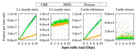
Fig. 4: Caches' features per time unit as a function of the input rate for CBR/Poisson traffic of 64B packets and CBR traffic of IMIX packets in *fastclick*.
