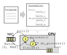
Fig. 2: The CPU is executing some instructions as a result of the translation from a high-level programming language.
