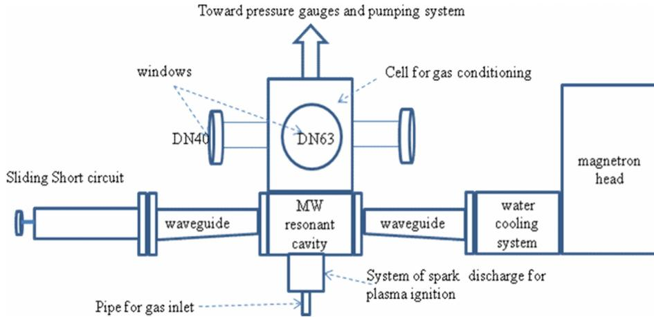
**Fig. 1. Schematic view of the experimental setup including the microwave resonant cavity with gas conditioning cell and the 2.45GHz microwave generator with a magnetron head and a power supply not shown in this scheme**
