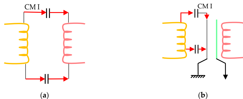
Figure 9. Correlation of CM current displacement across a transformer: (a) Standard unshielded transformer; (b) transformer with grounded electrostatic screens.
