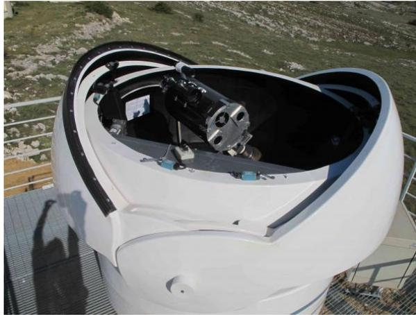
Figure 2. GDIMM instrument installed on the Calern Observatory.
