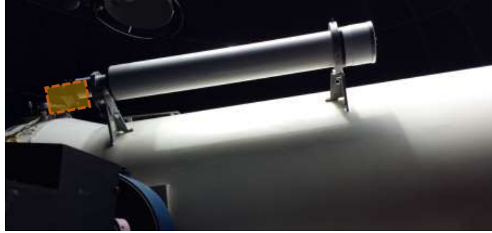
Figure 6. Wide filed Camera ( 1760 \times 2200 arcsec 2 Field of View) installed on 200 mm telescope mounted on MeO telescope.
