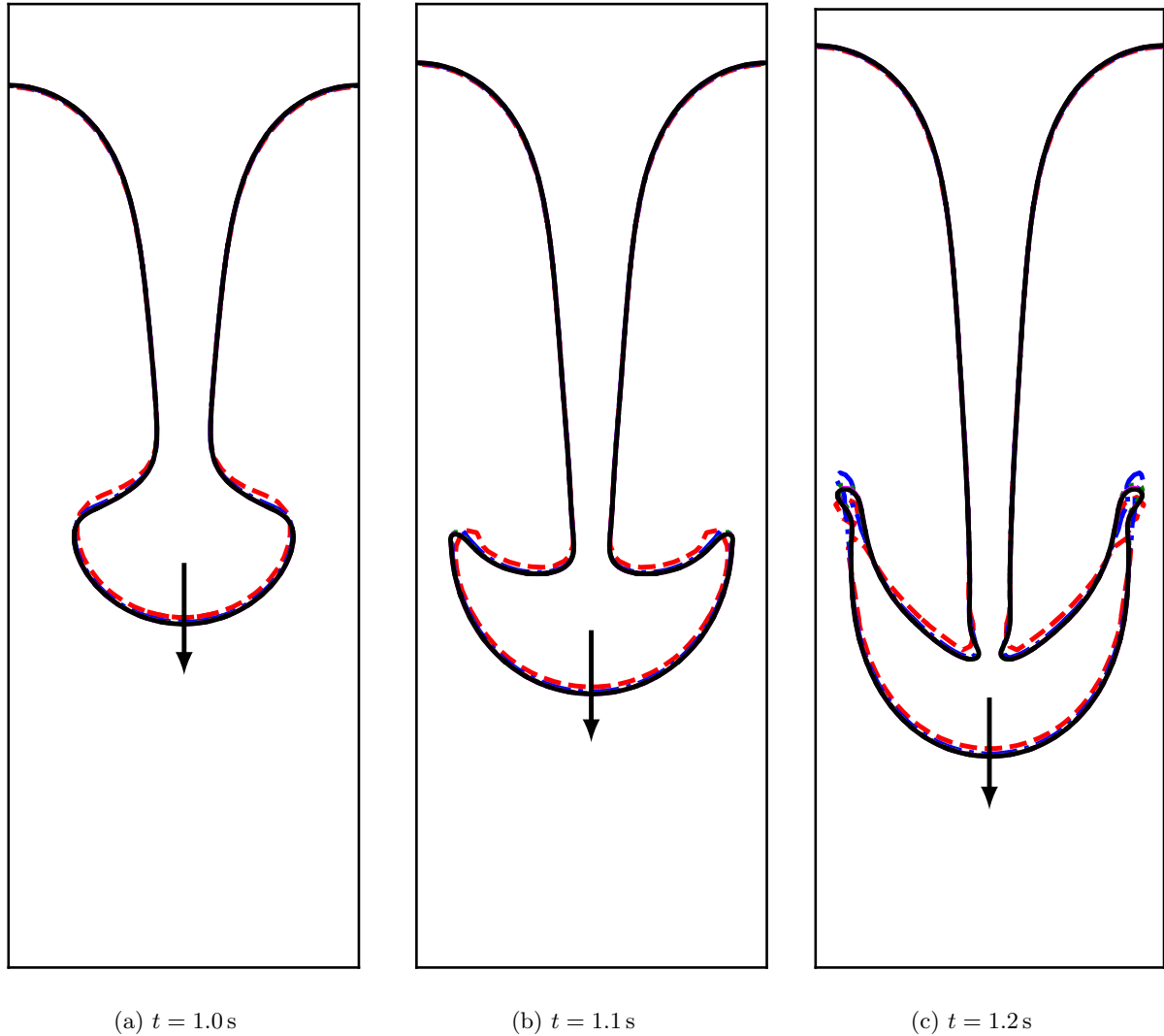
Figure 30: Overlap of phase interfaces for various mesh resolutions for Rayleigh-Taylor instability using HyMOFLS method. Arrow indicates increasing mesh resolutions from 32 \times 128 (---), 64 \times 256 (-.-.-), 128 \times 512 (.....), 256 \times 1024 (-.-.-), to 512 \times 2048 (—).
