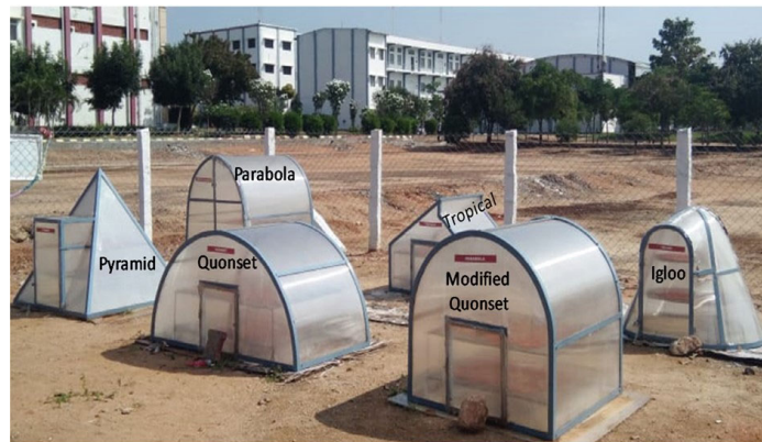
Figure 7. Photo of different shapes of passive SGHDs proposed in ref. [91] (adapted with permission).
