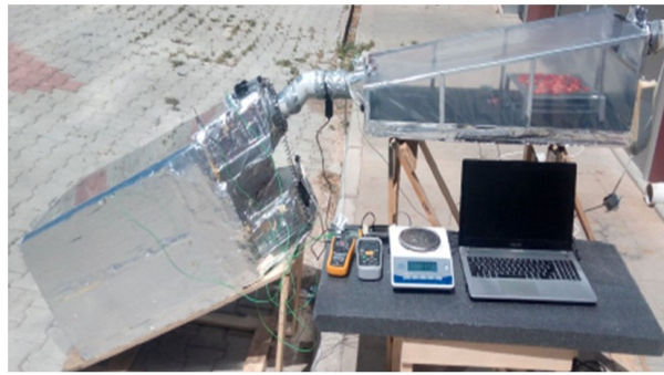
Figure 17. Experimental setup of the QPSAC integrated with a GHD, adapted with permission from [104].
