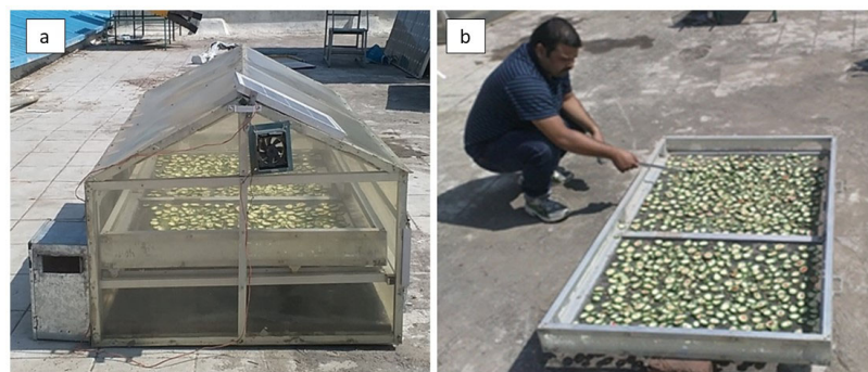
Figure 19. (a) Experimental setup of the GHD integrated with a solar thermal collector, under the forced convection, and (b) open-sun-drying, adapted with permission from [107].
