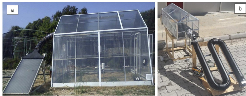
Figure 20. (a) Photo of the developed SGHD in ref. [28] (adapted with permission), and (b) tube-type solar air heater integrated with the GHD, adapted with permission from [108].
