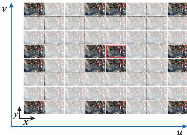
Fig. 3: Sparse representation of the  $8 \times 8$  LF image in subaperture representation with 16 reference views including the center view highlighted in red.
