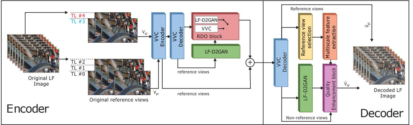
Fig. 5: Overall scheme of the proposed coding solution.
