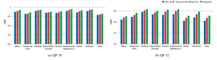
Fig. 11: SSIM performance of three LF image coding methods for the 9 considered test LF images at two QP values.
