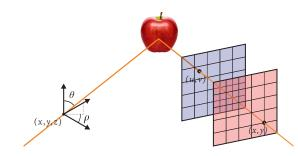
Fig. 1: 5D Plenoptic function on the left versus two-plane parametrization on the right (4D LF function).
