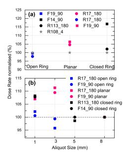
**Figure 3.** Experimentally determined normalised beta-dose rates. (a) Dose rate normalised to the respective fg value (sample R108\_4) versus beta-source shape; aliquot size is 7.95 mm (R17\_180; F19\_90) or 5 mm (F14\_90). (b) Dose rate normalised to 7.95 or 5 mm aliquot size plotted versus aliquot size. For the sake of clarity, error bars are not plotted. For data and uncertainty, see Table 3.
