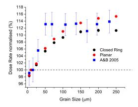
**Figure 5.** Result from *GEANT4* simulation compared to published experimental data. The dose rate is plotted as a function of grain size for the planar source and the closed-ring source and for experimental data (A&B 2005; Armitage and Bailey, 2005). Simulated data are normalised to the 10  $\mu$ m grain size; aliquot size is 7.95 mm on stainless steel cup. Experimental data of A&B 2005 are normalised to the 15  $\mu$ m grain size with aliquot size of 9 mm on aluminium disc.
