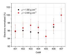
**Figure 9.** Result from *MCNP6* simulation: the number of electronproducing interactions plotted against cell number. The cell is a rounded SiO<sub>2</sub> grain of 300  $\mu$ m diameter of the two densities displayed. Data are normalised to cell no. 407, which is the grain surrounded by other grains (for spatial arrangement of cells, see Fig. 2b).
