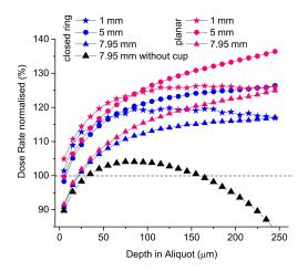
**Figure 7.** Result from *GEANT4* simulation: charge build-up in quartz grains of  $250 \,\mu\text{m}$  size resting on a 7.95 mm ss cup compared to no cup as a function of depth in the sample for the two beta-source geometries. The sample is composed of  $10 \,\mu\text{m}$  thick cylinder-shaped layers (see Fig. 1). Dose rate is normalised to the  $10 \,\mu\text{m}$  layer and 7.95 mm aliquot size and represented in percent.
