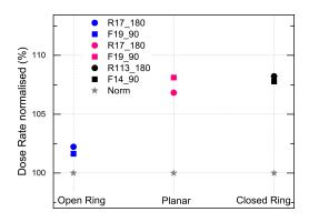
**Figure 4.** Beta-dose rates of 1 mm aliquots normalised to the 7.95 or 5 mm aliquot size of the respective sample versus beta-source shape. For the sake of clarity, error bars are not plotted. For data and uncertainty, see Table 3.
