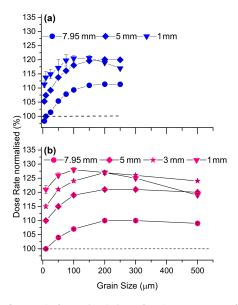
**Figure 6.** Result from simulations for dose rate as a function of grain size and aliquot size. Dose rate is normalised to the  $10 \,\mu m$  grain size and 7.95 mm aliquot size expressed in percent; (a) *GEANT4* for the closed-ring beta source; (b) *MCNP6* for the planar beta source and grain sizes up to 500  $\mu m$  to assess the significance of the trend.
