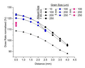
**Figure 8.** Result from *GEANT4* simulation: dose rate versus distance from centre of the stainless-steel cup for the closed-ring beta source. Data are for large (7.95 mm), medium (5 mm) and small (1 mm) aliquot sizes and for 10, 100, 200, and 250  $\mu$ m grain sizes. Dose rate is normalised to 10  $\mu$ m grain size, the average value of which is at 100 %.
