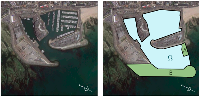
Fig. 3 Illustration of La Turballe port. Left : The port in its initial state. Right : The port with the two additional structures considered in this study: mole A and jetty B.
