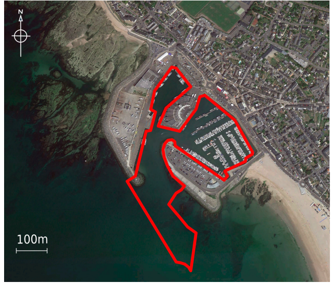
Fig. 9 The inner border (red) of the optimal configuration of the port, resulting from the minimization of energy. We observe an extended jetty and a wide mole.
