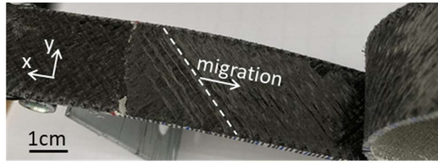
Fig. 13. Fracture surface of a DCB sample with +45^\circ// -45^\circ interface: observation of the delamination migration from one layer to the other.
