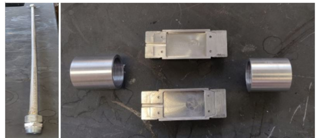
Figure 9: Drillstring components, Drillpipe (left), BHA components (right), from [14].
