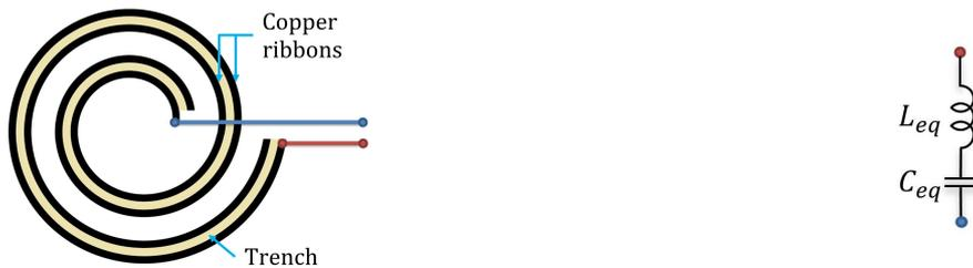
**Fig. 6** Use of a device as an LC series resonator. Left: top view of the copper ribbons (black), their connections (red and blue), and the trench (yellow); right: equivalent circuit.
