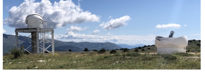
Figure 3. Calern Atmospheric Turbulence Station (CATS). On the left the GDIMM installed on a 4m tower, on the right the PML instrument observing the Sun limb.
