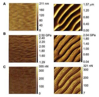
**Figure 7.** AFM quantitative nanomechanical measurements performed in a PeakForce QNM mode on  $azoCO_2Me$  thin film (thickness 300 nm) subjected to interferential illumination at 488 nm (240 mW cm<sup>-2</sup> each beam, p-polarized beams, 1  $\mu$ m periodic spacing): A) topography; B: Young's modulus E; C) adhesion. Left views: regular SRGs before superstructuration. Right views: area of superstructures after SRG superstructuration.
