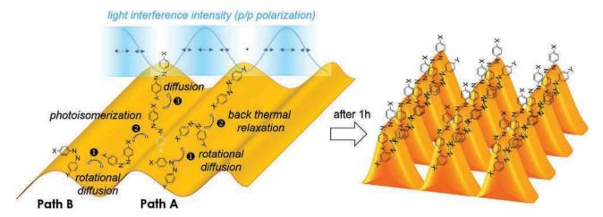
**Figure 10.** Schematic description of the envisioned thermal diffusion and back thermal relaxation leading to the rise of superstructures after long-time p/p polarized illumination.
