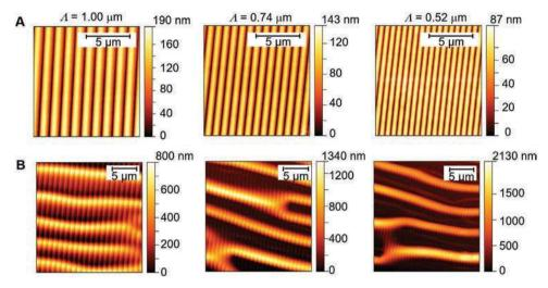
Figure 6. AFM images of azoCO<sub>2</sub>Me thin films subjected to interferential illumination at 488 nm (240 mW cm<sup>-2</sup> each beam) as a function of the periodic spacing of the light interferences (1.00 (left), 0.74 (middle), and 0.52 (right)  $\mu$ m). A) +45°/-45° polarization configuration (2 min irradiation). B) p/p polarization configuration (60 min irradiation).
