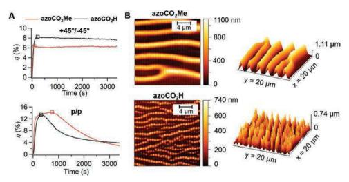
Figure 4. A) Time evolution of the first-order diffraction efficiency η of  $azoCO_2Me$  (red curve) and  $azoCO_2H$  (black curve) thin films subjected to +45°/-45° (top) and p/p (bottom) interferential illumination at 488 nm (240 mW cm<sup>-2</sup> each beam). Diffraction efficiency maxima are indicated by empty squares. B) AFM imaging (2D and 3D views) of  $azoCO_2Me$  and  $azoCO_2H$  thin films after p/p interferential illumination at 488 nm for 1 h (240 mW cm<sup>-2</sup> each beam).
