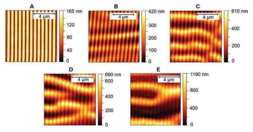
Figure 5. AFM imaging of  $azoCO_2Me$  thin film subjected to interferential illumination at 488 nm with a p/p polarization configuration (240 mW cm<sup>-2</sup> each beam,  $\Lambda = 0.74 \, \mu m$ ) after irradiation for: A) 2, B) 8, C) 15, D) 30, and E) 60 min.
