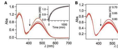
Figure 2. Spectral evolution of A) azoCO2Me and B) azoCO2H thin films (200 nm thickness) upon irradiation at 488 nm (7 mW cm-2) for 60 s (5 s time interval). Black arrows indicate the absorption change of films until reaching the photostationary state. Inset: back thermal relaxation in the dark (thick black) and biexponential fit (thin white) at the absorbance maximum 469 and 474 nm, respectively.
