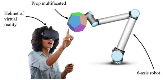
**FIGURE 1.** Conceptual scheme of the experimental platform
