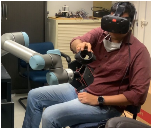
FIGURE 4. Human with HMD and hand tracker to control the movement of a UR 5 robot
