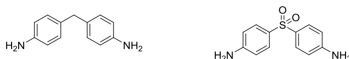
Figure 9: Telechelic diamine hardeners, 4,4'-diaminodiphenylmethane (DDM) and 4,4'-diaminodiphenylsulfone (44 DDS) used in the curing reaction 98
