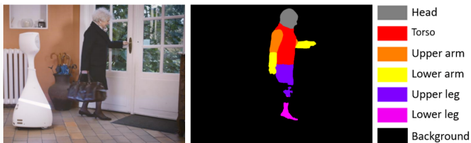
Fig. 3. Example of segmentation of the human body. Each part of the body is represented by a color, and the background in black. Each part of the body constitutes a distinct class.
