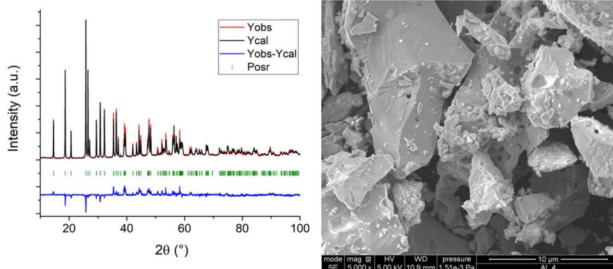
**Fig. 8** PXRD and SEM images of as-prepared brannerite sample. Observed, calculated, and the difference patterns after the Rietveld refinement of the crystal structure of brannerite (left panel), SEM image of the brannerite grains used for the dissolution experiments (right panel).
