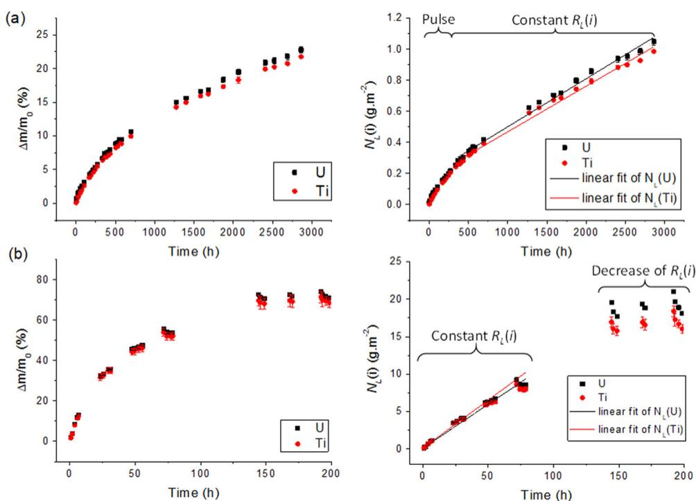
**Fig. 1** Released U and Ti during the dissolution of brannerite in 2 mol/L  $\text{H}_2\text{SO}_4$  with 2.8 g/L of Fe(III). Evolution of the relative mass losses  $\Delta m/m_0$  (%) and of the normalized weight losses  $N_L(i)$  ( $\text{g}/\text{m}^2$ ) obtained during the dissolution of synthetic brannerite samples in 2 mol/L  $\text{H}_2\text{SO}_4$  solution with 2.8 g/L of Fe(III) at 25 °C (a) and at 80 °C (b).
