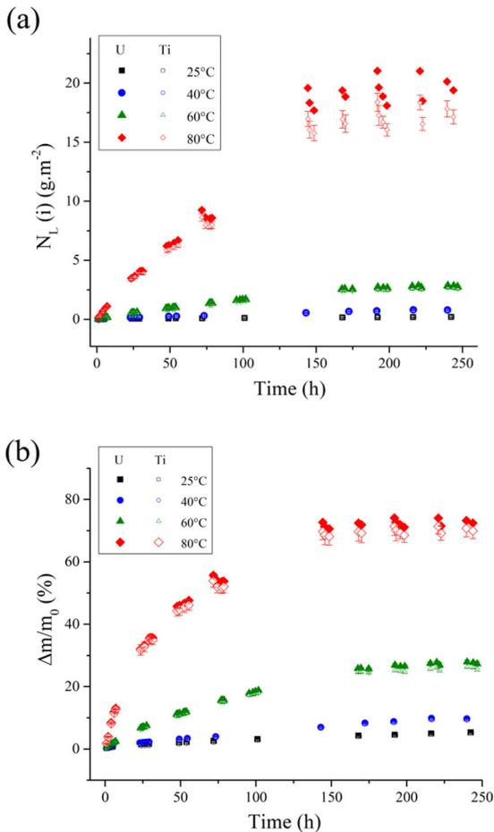
**Fig. 4** Dissolution of brannerite in 2 mol/L  $\text{H}_2\text{SO}_4$  with 2.8 g/L of Fe (III). Evolution of the normalized weight losses  $N_L(i)$  ( $\text{g}/\text{m}^2$ ) (a) and of the relative mass losses  $\Delta m/m_0$  (%) (b) obtained during the dissolution of synthetic brannerite samples in 2 mol/L  $\text{H}_2\text{SO}_4$  solution containing 2.8 g/L of Fe(III) for various temperatures.
