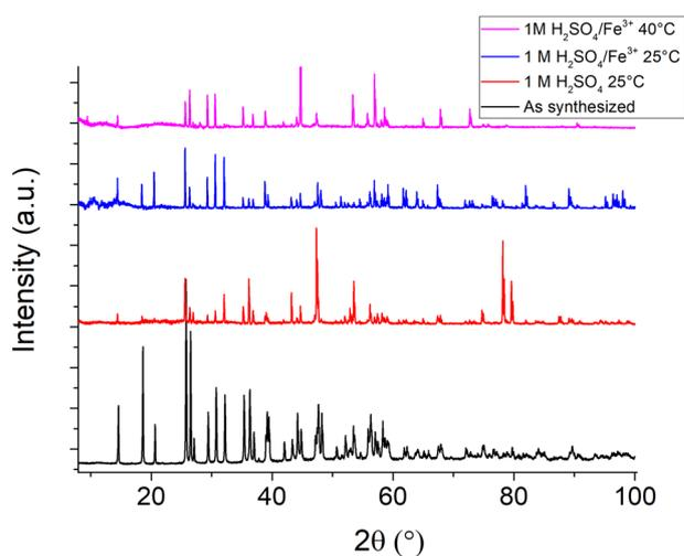
**Fig. 2** Powder X-Ray Diffraction (PXRD) patterns of dissolved brannerite samples. PXRD patterns corresponding to the brannerite samples obtained after leaching experiments labeled 2, 5, and 11 (see Table 3).
