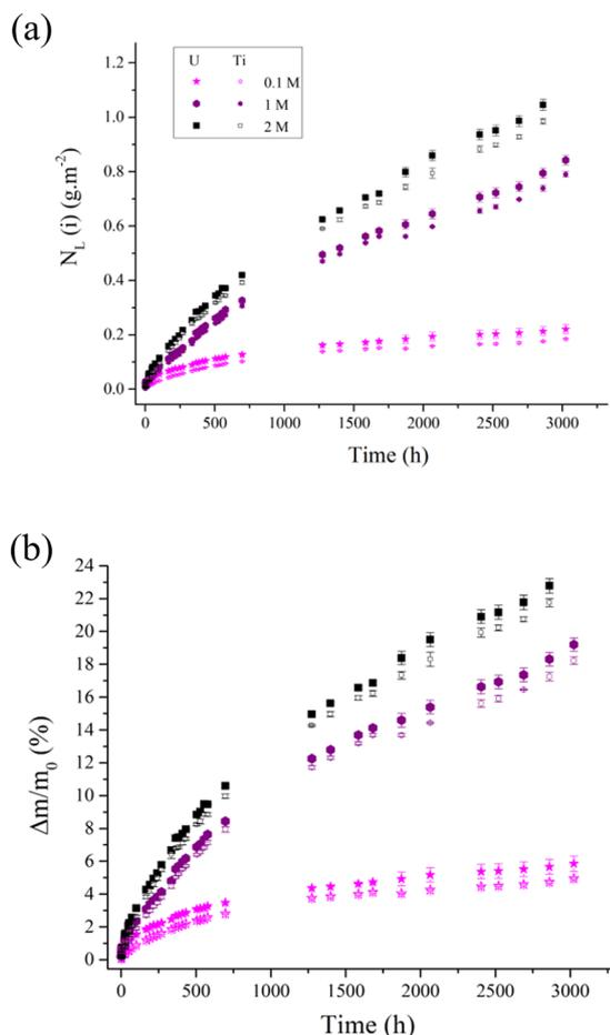
**Fig. 6** Dissolution of brannerite in  $\text{H}_2\text{SO}_4$  solutions with 2.8 g/L of Fe(III) at 25 °C. Evolution of the normalized weight losses  $N_L(i)$  ( $\text{g}/\text{m}^2$ ) (a) and of the relative mass losses  $\Delta m/m_0$  (%) (b) obtained during the dissolution of synthetic brannerite samples in various  $\text{H}_2\text{SO}_4$  solutions containing 2.8 g/L of Fe(III) at 25 °C.
