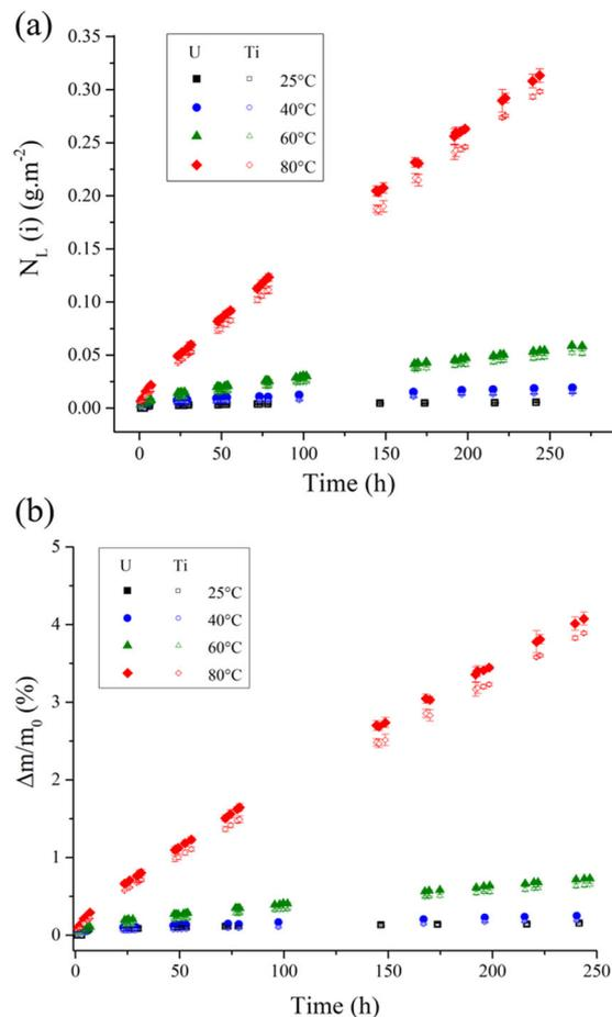
**Fig. 3** Dissolution of brannerite in 2 mol/L H<sub>2</sub>SO<sub>4</sub>. Evolution of the normalized weight losses  $N_L(i)$  (g/m<sup>2</sup>) (a) and of the relative mass losses  $\Delta m/m_0$  (%) (b) obtained during the dissolution of synthetic brannerite sample in 2 mol/L H<sub>2</sub>SO<sub>4</sub> solution for various temperatures.
