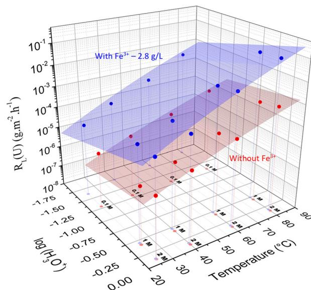
**Fig. 7** Experimental and simulated dissolution rates of brannerite. Simulated maps obtained by fitting the multiparametric expression of the normalized dissolution rate of synthetic brannerite samples based on the data obtained without (red dots) or with (blue dots) Fe(III) in sulfuric acid solutions.
