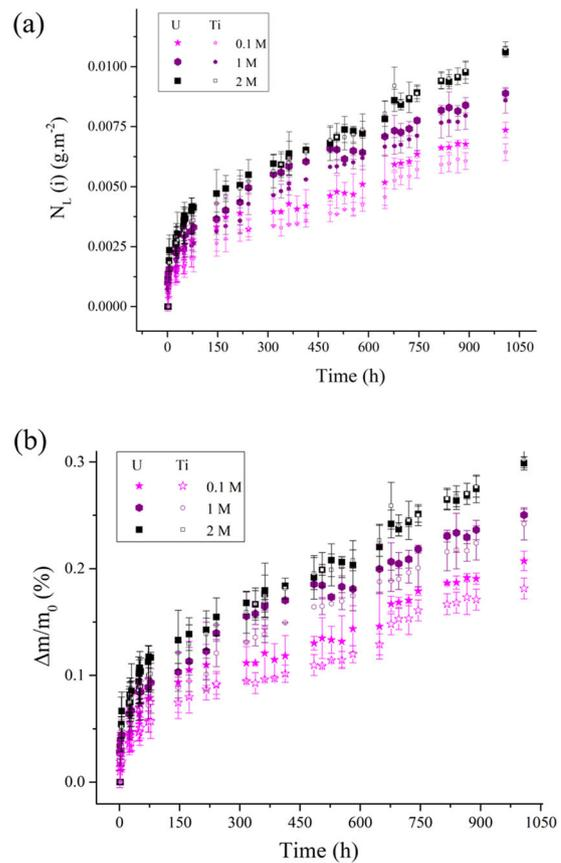
**Fig. 5** Dissolution of brannerite in  $\text{H}_2\text{SO}_4$  solutions at 25 °C. Evolution of the normalized weight losses  $N_L(i)$  ( $\text{g}/\text{m}^2$ ) (a) and of the relative mass losses  $\Delta m/m_0$  (%) (b) obtained during the dissolution of synthetic brannerite samples in various  $\text{H}_2\text{SO}_4$  solutions at 25 °C.
