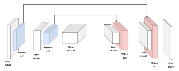
Fig. 2. Our proposed DCSNN architecture. White, blue and red cubes represent LIF convolutional layer, maxpool layer, and upsampling layer respectively. Black arrows are residual connections between feature maps (i.e. addition operations). For simplification purposes, the readout linear layers (specific to DECOLLE [9] model) are not shown.
