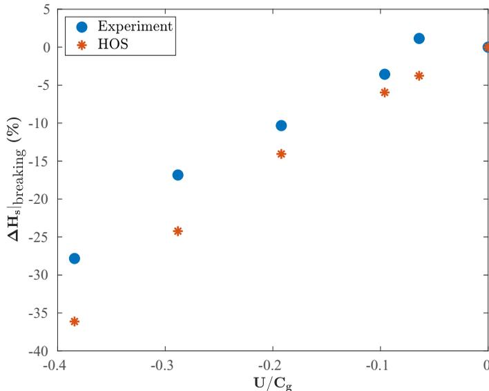
FIG. 5. Energy loss due to wave breaking.
