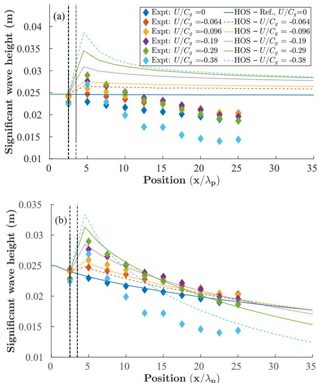
FIG. 4. Evolution of significant wave height  $H_s$  as a function of the nondimensional distance  $x/L_p$  from the wave maker for different current speeds: (a) without and (b) with wall friction dissipation. Marks indicate experimental observations, the solid lines refer to numerical simulations, and the dashed vertical lines indicate the start and end of the transition region from no current to regime flow.
