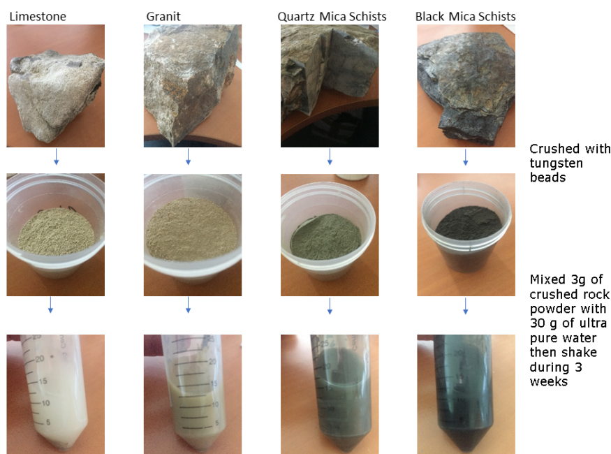
Figure 3. Rock leaching experimentation.
