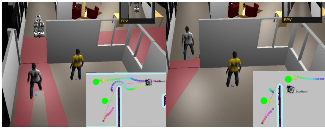
Fig. 3: Door crossing scenario in the simulated environment. The human moves towards the door. The robot sees the human and waits on the side of the door (right) until the human crosses.
