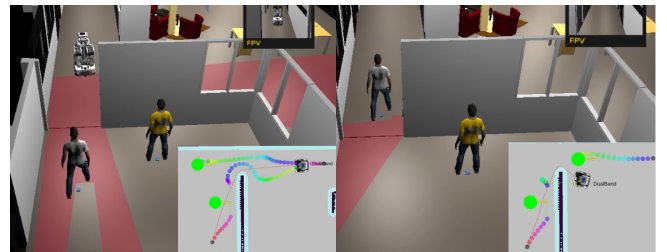
Fig. 3: Door crossing scenario in the simulated environment. The human moves towards the door. The robot sees the human and waits on the side of the door (right) until the human crosses.
