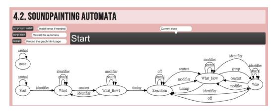
Figure 4. Finite-state automaton representing the grammar for the "default mode" of Soundpainting. The graph shows the different states of the automaton and the possible transitions between them.
