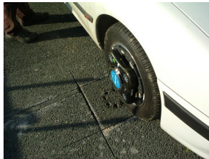
Figure 2. The Kistler wheel on the MEVI system [6]
